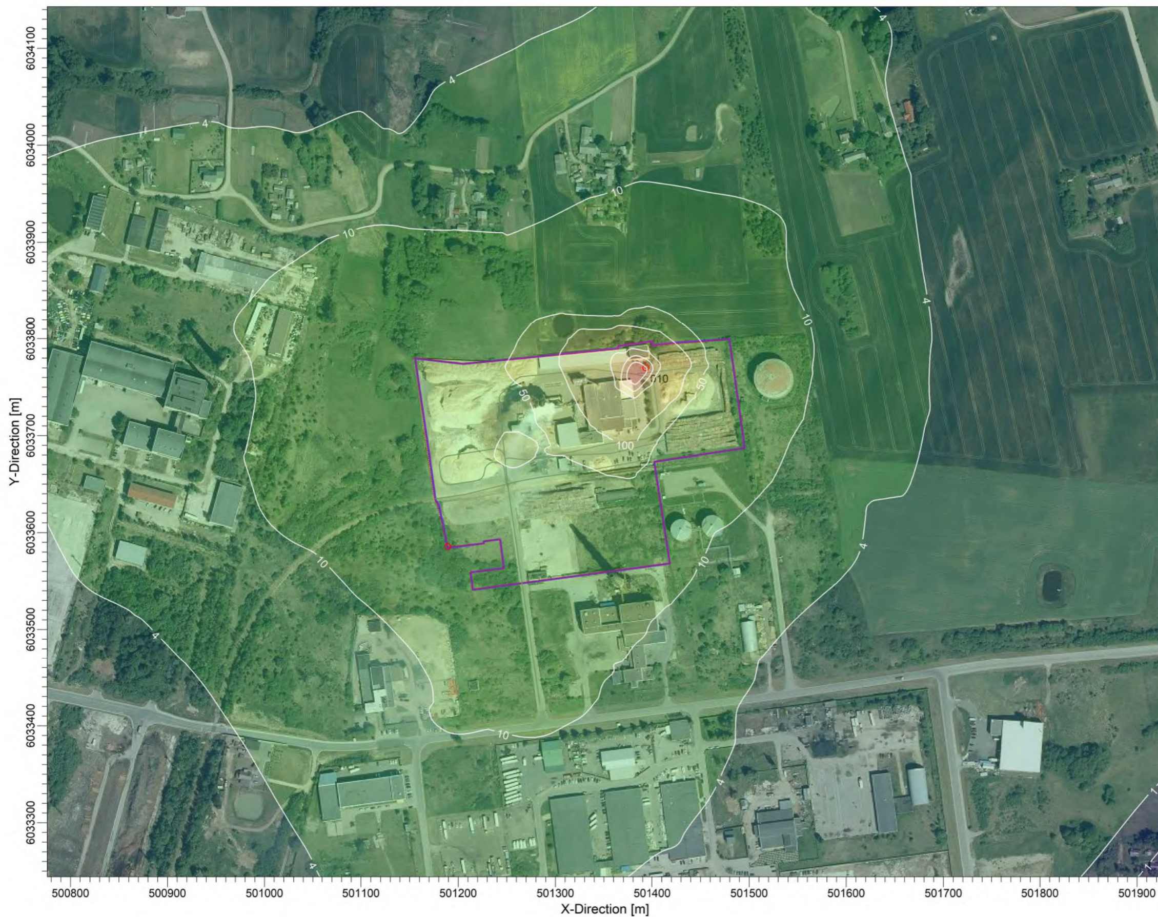
PLOT FILE OF 98.50TH PERCENTILE 1-HR VALUES FOR SOURCE GROUP: IMONEMOB Max: 2333 [ \mu\text{g}/\text{m}^3 ] at (501383,24, 6033764,46)
