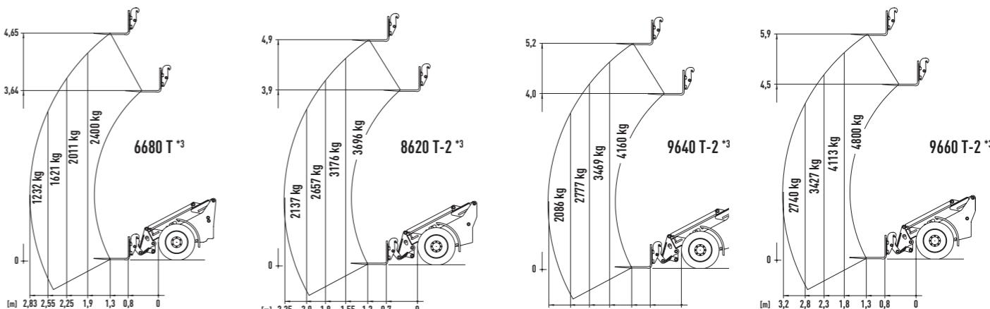
\*1 boom horizontal, not extended, with pallet fork [acc. to ISO 14397] \*2 according to ISO 8041 \*3 using forks on stable underground (according EN 474-3)
